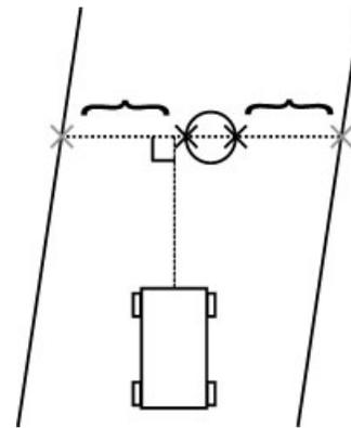
**Figure 8.** Corridor gap geometry. Black x’s mark unpaired endpoints; gray x’s mark corridor endpoints; and braces show the resulting corridor gaps.
