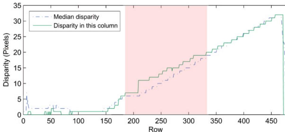
**Figure 4.** Disparity values and obstacle detection in the highlighted column of Figure 3(a). The shaded region is detected as an obstacle.
