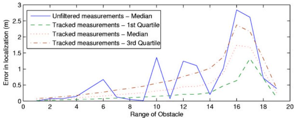
Figure 6. Error in localization versus range in meters.
