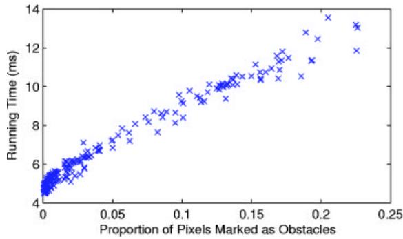
**Figure 5.** Computation time versus proportion of obstacle pixels over 193 640 × 480 images.
