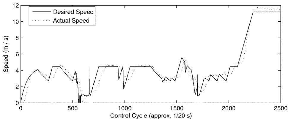
Figure 2. Speed versus time at start of NQE Run 1.
