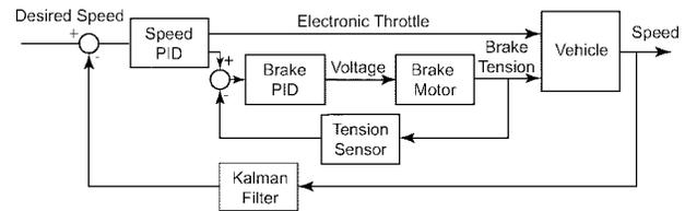
Figure 1. Speed control functional block diagram.
