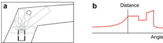
**Figure 7.** (a) A sample world configuration consisting of GPS course boundaries, a circular obstacle, and the vehicle. Projected tubes are shown in gray. (b) The resulting polar tube plot.
