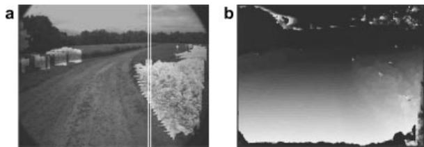
**Figure 3.** (a) Sample scene image, with detected obstacle pixels highlighted and sample column outlined, as analyzed in Figure 4. (b) The corresponding disparity map.
