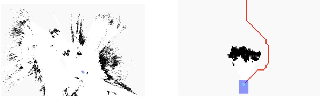
(a) A cost map generated from stereo vision data (b) A path planned through a cost map
